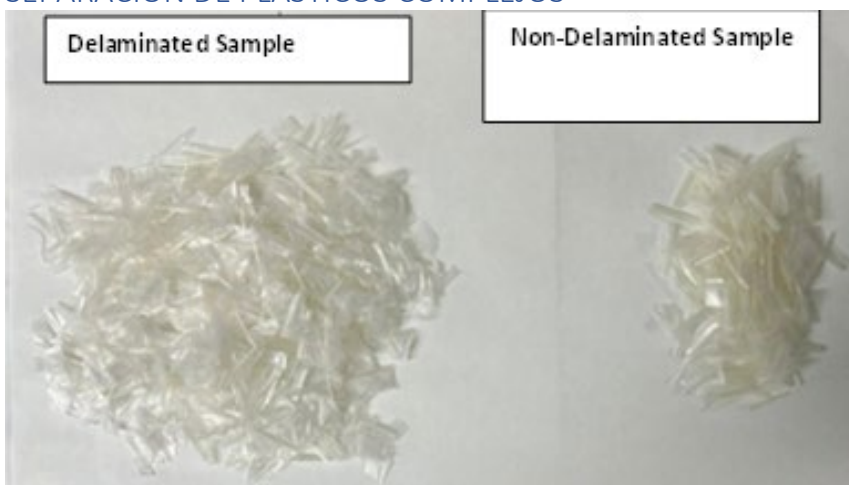
Figure 1. Example of delaminated sample with MANDALA DAF adhesive: PEF//rLDPE 89% delamination. Video complete: https://www.youtube.com/watch?v=IW2XRFhD1fo
